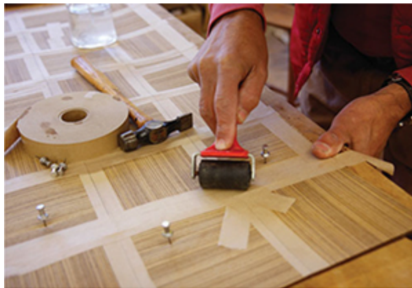
A roller secures the veneer tape and ensures a strong bond and a tight seam.
