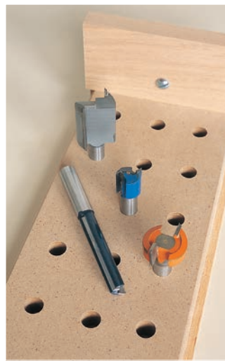
An ordinary straight bit is fine for cutting laps with the sliding fence. Use the largest diameter straight you have. Even better is a mortising bit. Another option for end laps is a long straight bit. Again, a large diameter bit is better than a small one.
