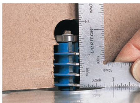
The solid finger-joint bit is tricky to adjust the first time you use it. Try this: elevate the cutting edges above the table, then lower the bit until the bottom-most finger cutter is just 1/16" above the table. The initial test cut (right) will have a finger on the bottom.
