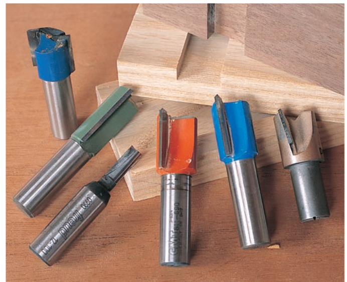
The range of bits that can cut dadoes and grooves is almost endless. Use the shortest, heaviest-shanked bit that will produce the desired cut. For veneered materials (like plywood), a downshear bit (right) is least likely to chip the edges.
