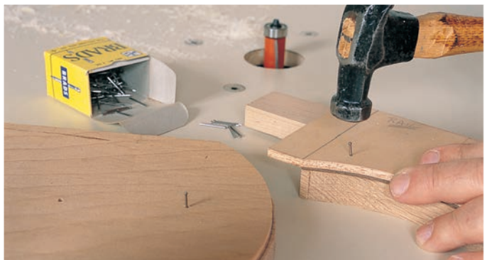
If the template will be on top and tiny holes in the work don't matter (for example, they'll be hidden inside an assembly), you can use small nails or brads to fasten a template and workpiece together.
