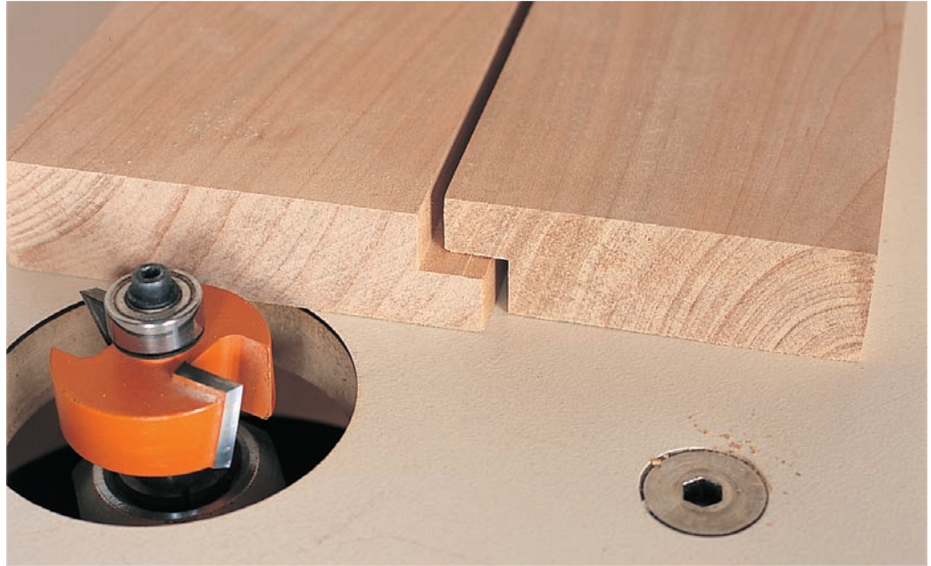
A shi lap joint is formed by overlapping rabbets cut into opposite faces of adjoining boards. The rabbets are quickly cut, precision is irrelevant, yet they serve a valid purpose.
