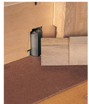
Cut the lap with the piece on end and backed up with a scrap pusher. The lap, straight from the cut, is smooth and will glue exceptionally well.
