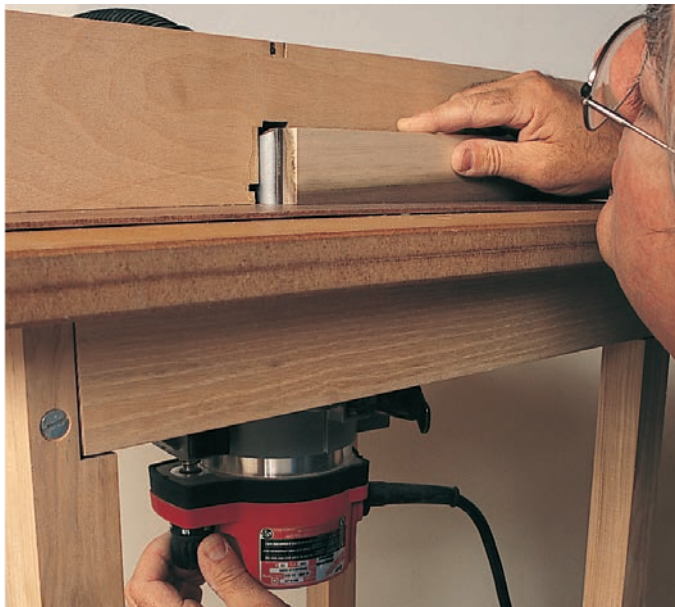
A half-lap can be cut with a very long straight bit, if you have one. Lay a part to be lapped beside the bit and adjust the bit extension to match its width.
