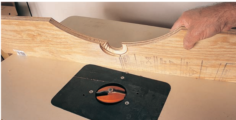
A fence doesn't have to be straight. This job-specific fence was made to safely raise the arched tops of a big batch of panels. The curve was cut with a router and trammel and the cutout for the pilot was bored with a Forstner bit. Except at the beginning and end of each cut, the bit is shrouded by the panel and the fence.
