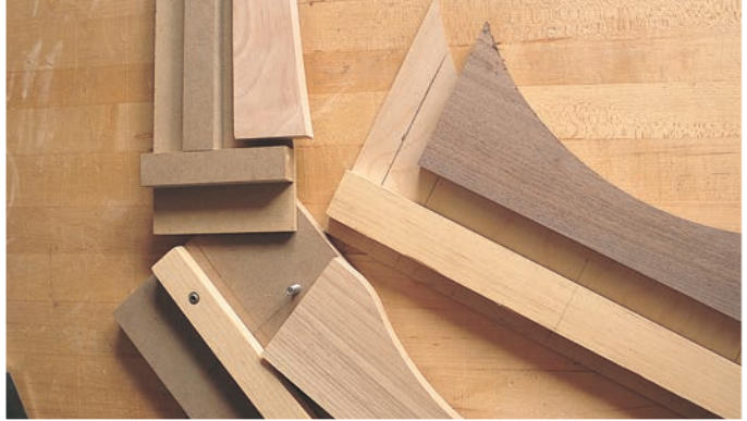
A fence or two ensure that each part is identically shaped. The template at upper left has fences to position the blank in relation to the contoured edge as well as trap the ends. At right is a template with only one fence; each workpiece must be aligned with penciled lines. The third template has a fence, but pins trap the ends of the blank.
