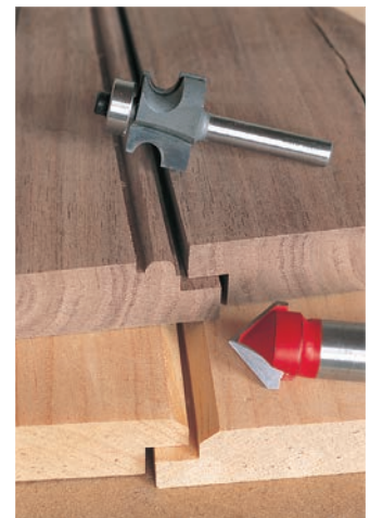
A shi lap joint is formed by overlapping rabbets cut into opposite faces of adjoining boards. The rabbets are quickly cut, precision is irrelevant, yet they serve a valid purpose.
