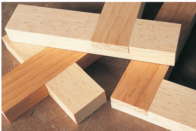
A half-lap joint is strong, versatile, and easy to cut. To make one, you cut recesses in both mating pieces, then fit them together, forming an X, L, or T.
