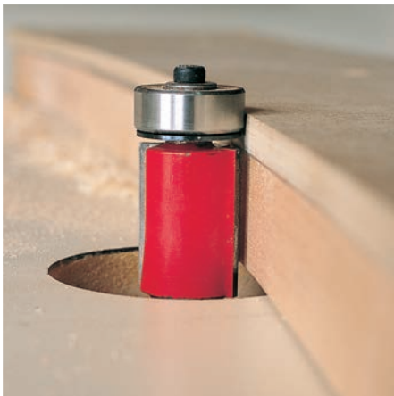
Flush-trimming bits (left) and pattern bits (right) are used for template work on the router table. You can get either type in a wide variety of lengths and diameters.
