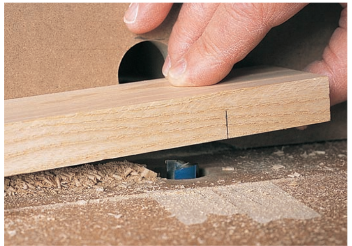
Begin a blind groove with the trailing end of the work resting on the table and the leading end tipped up above the bit (left). Align the mark on the workpiece with the tape marking that will place the bit inside the groove. Plunge the work down onto the bit and advance it until the end mark aligns with the other tape mark. Tip the work up off the bit (right).
