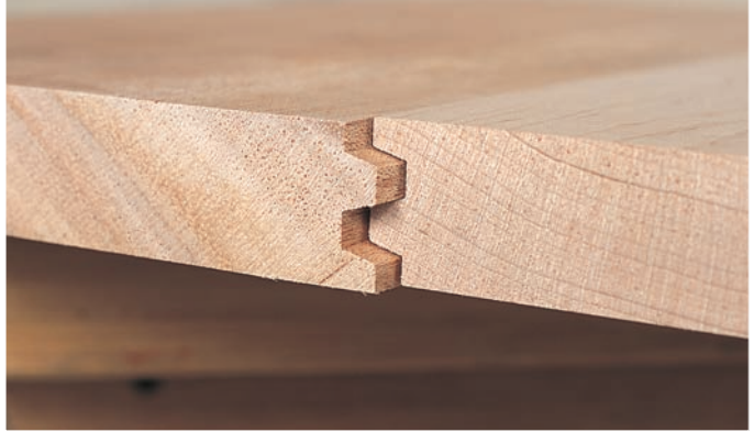
The glue joint is perfect for edge joining multiple boards because it's self-aligning. Simply add glue and clamp the assembly together.
