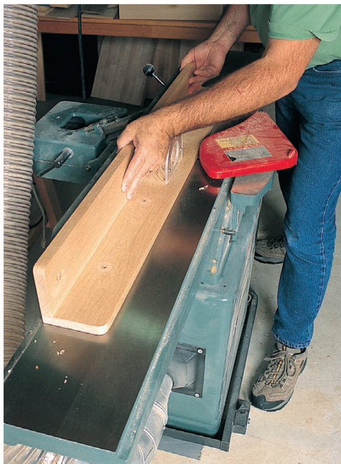
A wooden fence with no fasteners or hardware can be jointed to true it. Run the base surface across the machine to flatten it. When the base is flat, hold it tight to the jointer fence and feed it across the knives to flatten the fence face and square it to the base.
