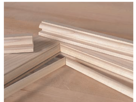
Make profiled retainers for your glazing by sticking the edges of narrow strips, then ripping the profile free. Miter the ends and glue them into the frame to secure the glass panes.
