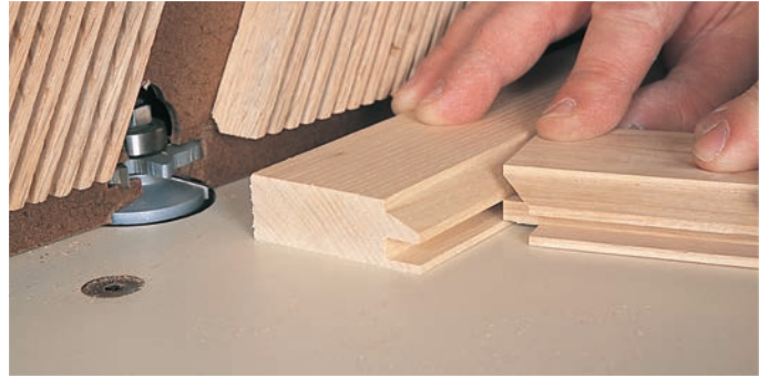
Cut quickly with specialized router bits, the cope-and-stick joint looks great and is strong enough for cabinetry applications. The nature of the joint gives you great latitude to adjust the position of the rail along the stile.
