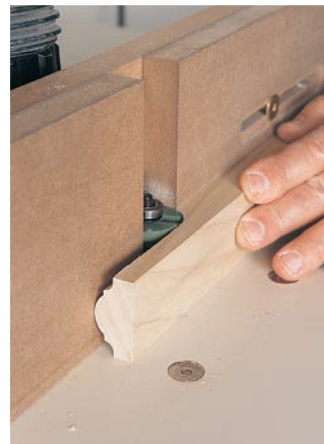
Routing a profile into the face of a board isn't easy if you depend on the pilot to control the cut. But with the fence controlling the cut, you've got support for the board, and the operation is safe and trouble-free. And you get the profile where you want it.
