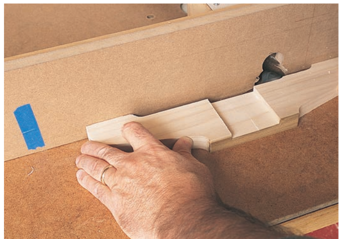
Creating a relief in the bottom of a trestle foot is a simple blind cut. But making feet for a team of shop horses means routing the same cut in piece after piece. Marks on the fence delineate where the foot must align to begin and end the cuts. Line up the toe with the starting line, push the foot against the fence. Feed until the heel lines up with the finish line and pull the foot away from the fence.
