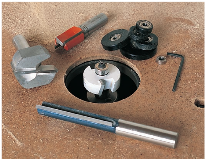
A rabet bit with set of interchangeable pilot bearings sets up quickly and produces a variety of specific-width rabbets. Straight bits you may already have and use for other cuts will also produce rabbets on straight stock. A mortising bit, effectively a rabet bit without the pilot, also cuts clean rabbets.
