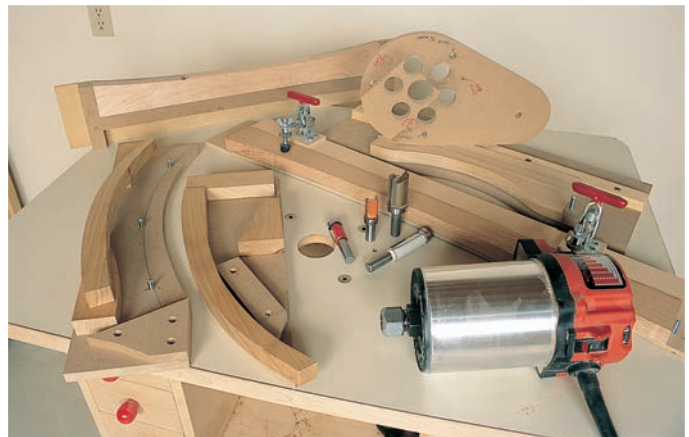
Templates play a key role in creating all sorts of parts for woodworking projects. The template-guided cut is often easier to make on the router table than with the router hand-held.
