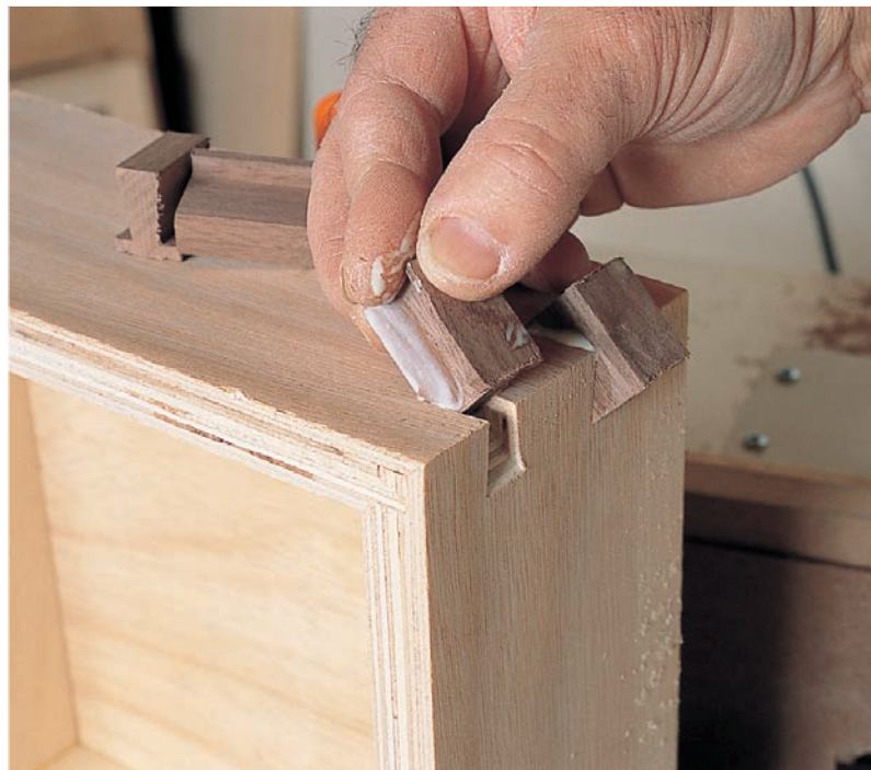
Cut your key strips into short keys, then glue a key into each slot. Clamping isn't necessary.
