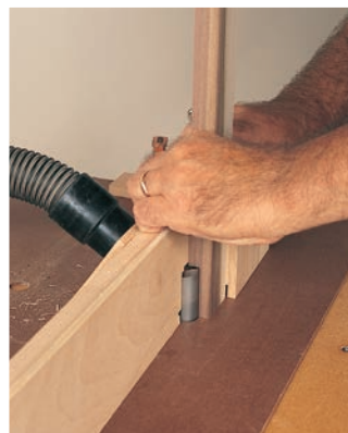
Cut the lap with the piece on end and backed up with a scrap pusher. The lap, straight from the cut, is smooth and will glue exceptionally well.
