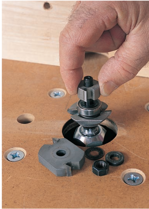
Cut joinery for rabbeted frames with a common pair of cope-and-stick bits. Remove the slotter from the cope bit and replace it on the arbor with a sleeve-type spacer or a stack of washers. A cut with it will produce a cope and a blocky tenon to fill the rabbet.
