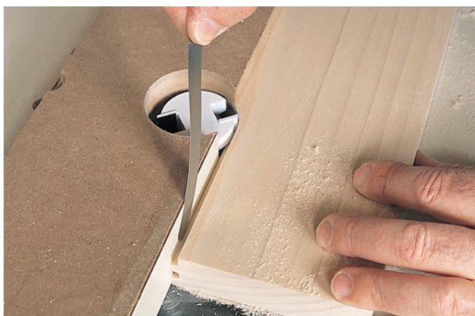
Check the fence setting next. Cut several inches of a stock sample and stop. If the fence position is correct, as it is here, both the cut and uncut edges will be in contact with the fence. If there's any gap between the cut edge and the fence (even a paper-thin one), the fence must be inched back to eliminate it. If the fence is too far back, the sample hits the edge of the outfeed fence facing.
