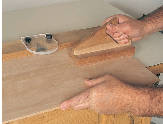
Profiling wide strips and raising panels calls for a pusher that applies pressure over a broad area. This shop-made float-type has a tactile layer—cut from an old computer mouse pad—glued to the sole.
