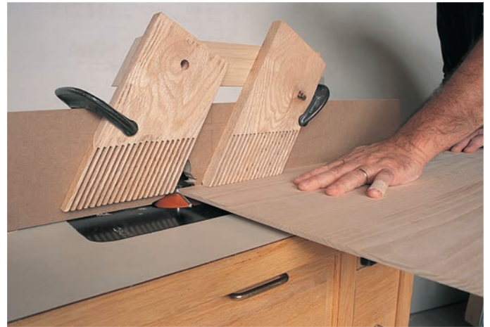
The proof of your setup is in the fit of the panel to its groove in the frame. Make a cut on a sample of the panel stock and fit it to an actual frame member. The ideal is a snug press fit.
