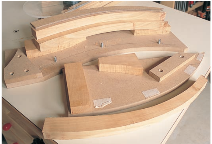
Continuous fences are sometimes more trouble than they're worth. Three or four contact points are usually all you need. On the concave-curve template (at top of photo), the blank butts against the base fence and its convex edge contacts just the corners of the MDF fence. On the convex-curve template (at bottom of photo), the blank fits against machine screws. Carpet tape secures the blanks.
