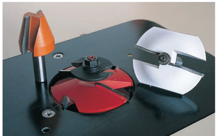
A panel-raising bit is serious business. The horizontal bit with an undercutter (center) is as big a cutter as a router can handle. In comparison, even a full-sized ( 3\frac{1}{2} "-diameter) raiser without the undercutter (right) seems somewhat smaller. Smallest are the vertical bits (left). The horizontal bits are more widely available than the vertical bits, and they are made in a much greater variety of sizes and profiles.
