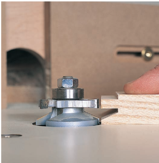
Adjust the elevation of the sticking bit using a rail as a gauge. Align the bit's slotter with the stub tenon.
