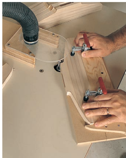
Templates play a key role in creating all sorts of parts for woodworking projects. The template-guided cut is often easier to make on the router table than with the router hand-held.
