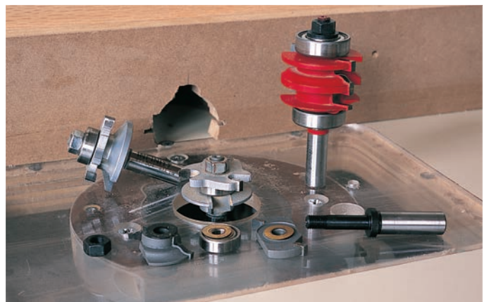
Three types of cope-and-stick cutters are (clockwise from the top) the matched pair, the stacked bit, and the assembly. All are available in several profiles: bead, quarter-round, ogee, cove-and-bead (sometimes called classical) and bevel (sometimes called traditional or straight). A 1\frac{1}{2} -hp router can drive these bits, and it can be run at full speed.
