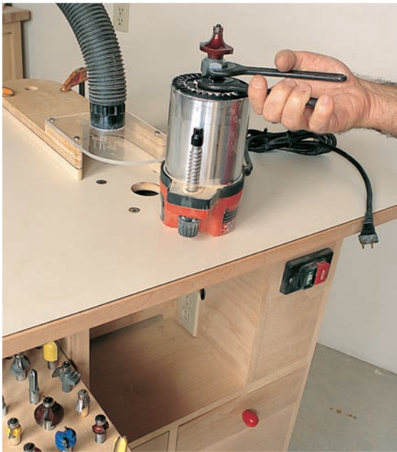
There's no reason why you have to leave the router in the table for bit changes. Pulling the router and mounting plate from the table, or just dropping the motor out of its base, has always been a sensible, convenient approach. With the tool on the tabletop, you have a clear view of the bit and collet and easy wrench access. In addition, it gives you an opportunity to check over the tool.
