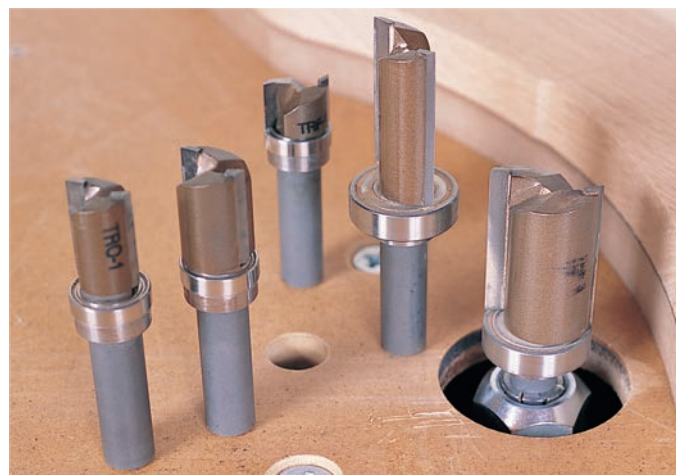
Any straight bit with a cutting diameter larger than its shank diameter has the potential to be a pattern or offset pattern bit. Slide a bearing onto the shank and secure it with a collar. A pattern bit needs a bearing matching the bit's cutting diameter. A bearing \frac{1}{8} " larger than the cut diameter makes an offset pattern bit.
