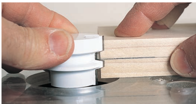
Set the gluejoint bit height by eye initially. Mark the center of the work, and align the sweet spot on the gluejoint bit with your mark. While the height probably won't be perfect, it'll get the setup process started.
