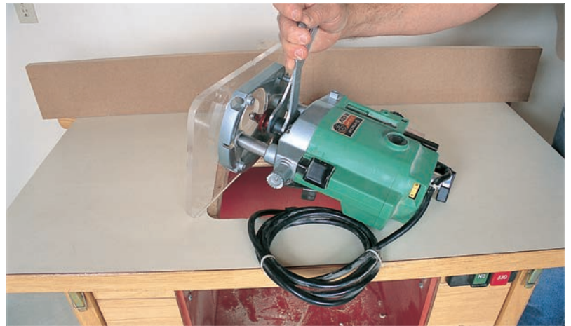
There's no reason why you have to leave the router in the table for bit changes. Pulling the router and mounting plate from the table, or just dropping the motor out of its base, has always been a sensible, convenient approach. With the tool on the tabletop, you have a clear view of the bit and collet and easy wrench access. In addition, it gives you an opportunity to check over the tool.
