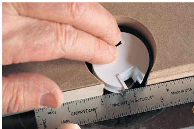
After shimming the outfeed half of the fence, align that side tangent to the cutting edges of the bit's smallest diameter. To find the correct alignment, use a straightedge and turn the bit by hand (unplug the router first). You want the cutting edge to graze the rule without actually moving the rule.
