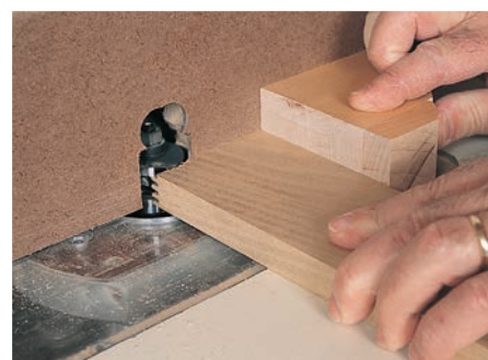
The finger joint is often used to assemble pieces end to end. Use a backup block as a pusher. It keeps the narrow workpiece from walking along the fence and it prevents splintering on the backside when the cutter breaks out of the cut.
