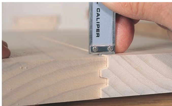
Cut a test joint. If the faces are flush, your setup is dead-on. If there's a step, measure it with the depth bar of a machinist's calipers. The adjustment to make is half the measurement.
