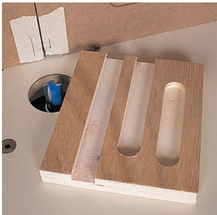
A through groove (left) extends from one end through the other. A stopped groove (center) begins at one end but stops short of the other end. And the blind groove (right) begins and ends short of either end of the workpiece.
