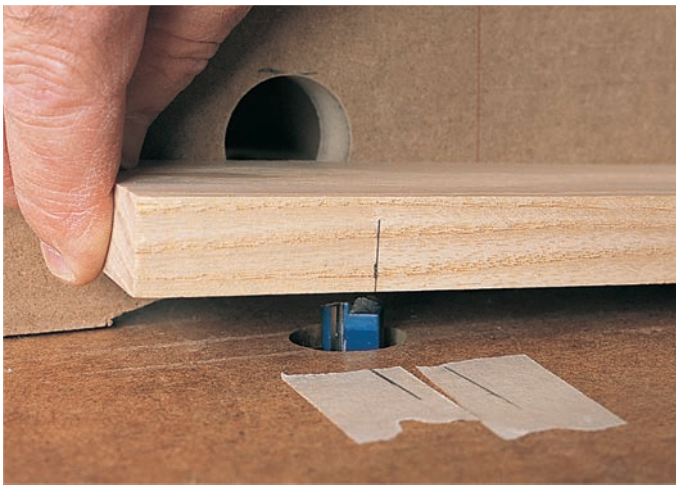
Begin a blind groove with the trailing end of the work resting on the table and the leading end tipped up above the bit (left). Align the mark on the workpiece with the tape marking that will place the bit inside the groove. Plunge the work down onto the bit and advance it until the end mark aligns with the other tape mark. Tip the work up off the bit (right).
