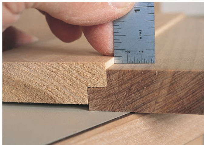
As a halving joint, the shi lap is easy (in concept) to fit. Cut a rabbet on a sample of the working stock, crosscut it and fit the joint together. If the pieces aren't flush, measure the offset with the depth bar of dial calipers. Raise or lower the bit by half the offset.
