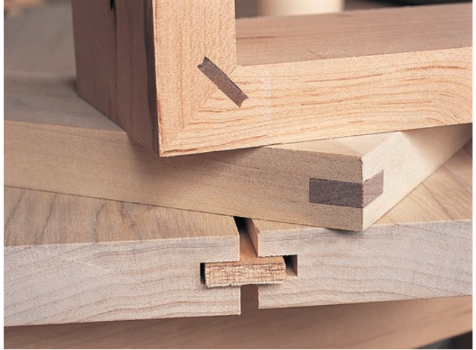
Splines are a great way to reinforce case miters (top), frame miters (center) and edge to edge joints (bottom). Rout the grooves for the splines on the router table.
