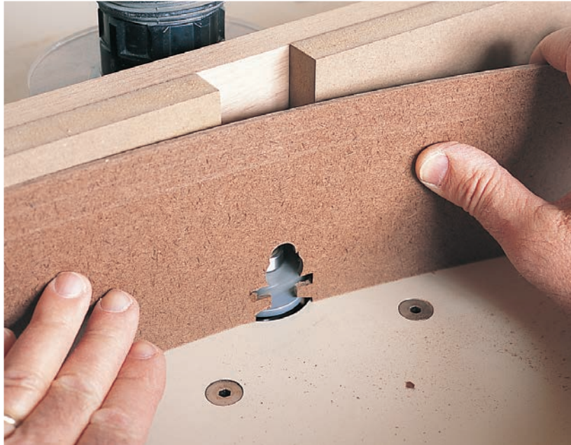
Use a thin hardboard or plywood facing for the fence, and cut a zero-clearance opening for the bit. Cut an initial opening for the bearing and arbor. Press the outfeed side against the fence, but flex the rest of the plywood and hold it clear of the bit. Switch on the router and roll the facing onto the fence, while the bit cuts through the edges of the opening. Then secure the facing with carpet tape or spring clamps.
