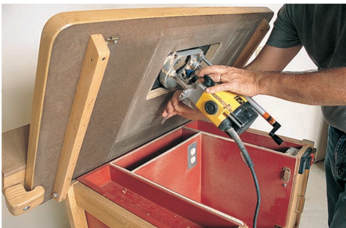
The tilting top gives you unfettered access to the router without having to remove it from its mounting. With a plunge router, back the motor down the posts to expose the collet, then use the wrenches. To expedite plunge adjustment, use a $35 crank instead of the more commonplace knob.
