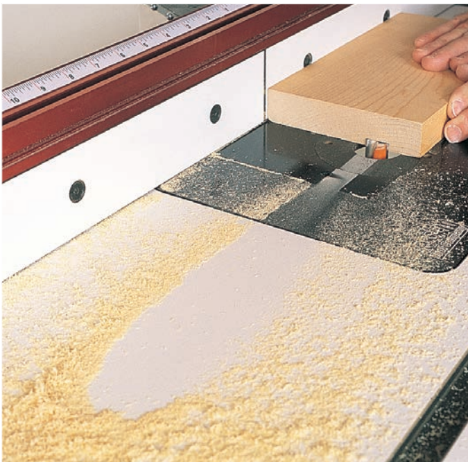
A simple grooving cut sprays dust out of the cut and across the table-top. The typical dust pickup on the table's surface may capture the dust, but it'll need to be in the cut path.
