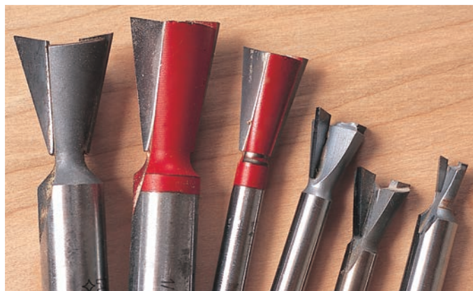
Dovetail bits are made in a wide variety of diameters, roughly from \frac{1}{4} " up to 1". Angles range from 7^\circ to 14^\circ .
