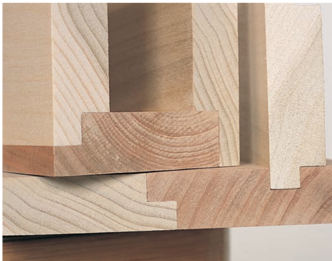
The rabet is the basis for a variety of joints, including the single rabet, the double rabet, the shiplap, and the dado-and-rabet.
