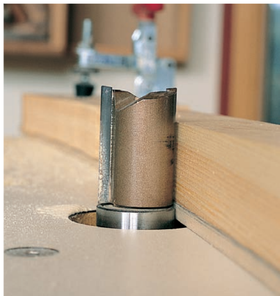
Flush-trimming bits (left) and pattern bits (right) are used for template work on the router table. You can get either type in a wide variety of lengths and diameters.
