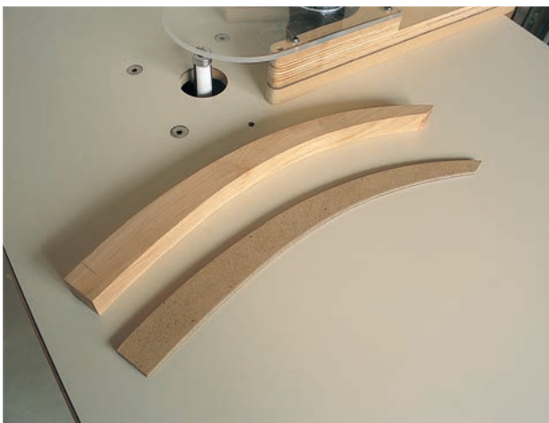
Making a batch of small parts safely often requires more than one template. The small curved slat shown (left) is a good example. The slat is too slender to be routed using a rout-around template. But you do need a pattern to lay out the slat blanks, and making that pattern from hardboard rather than cardboard simplifies making the working templates. Use it to make a convex template (center) and a concave template (right). Band-saw a slat blank and stick it to the convex template with carpet tape. Position fences—they need only contact the blank at three places to locate it—and attach them to the template. After shaping the blank's convex edge, stick it to the concave template. Mount fences (machine screws are used here) to locate the blank. Rout the concave edge. (The extra blocks attached to the templates are scraps of the working stock; they allow the templates to be inverted and used with a flush-trimming bit.)
