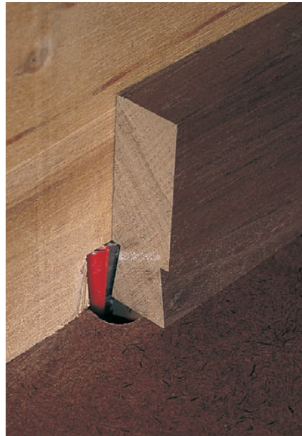
Dovetail keys are cut on the router table, usually using stock that contrasts with the box. Cut the key strips parallel to the grain of the stock.
