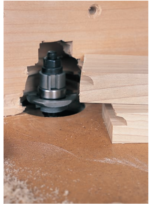
Cope the rail ends first, just as you do in making a wood-panel door with this joinery. Use a square-ended block to push the workpiece through the cut and to back up the good stock, so exit blow-out doesn't damage the frame part.
