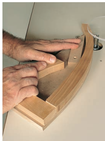
Making a batch of small parts safely often requires more than one template. The small curved slat shown (left) is a good example. The slat is too slender to be routed using a rout-around template. But you do need a pattern to lay out the slat blanks, and making that pattern from hardboard rather than cardboard simplifies making the working templates. Use it to make a convex template (center) and a concave template (right). Band-saw a slat blank and stick it to the convex template with carpet tape. Position fences—they need only contact the blank at three places to locate it—and attach them to the template. After shaping the blank's convex edge, stick it to the concave template. Mount fences (machine screws are used here) to locate the blank. Rout the concave edge. (The extra blocks attached to the templates are scraps of the working stock; they allow the templates to be inverted and used with a flush-trimming bit.)
