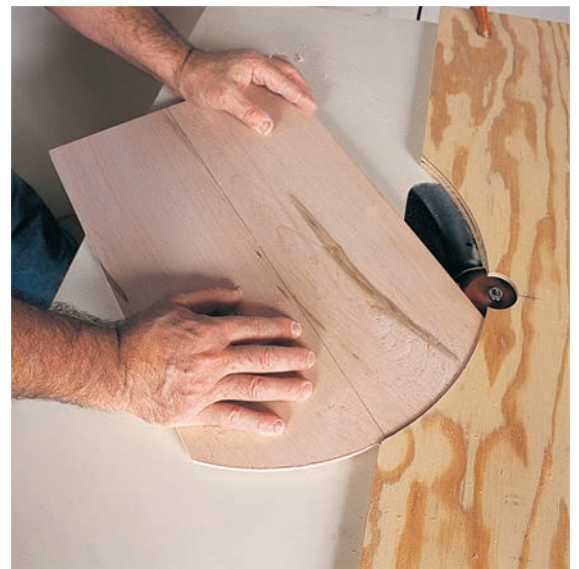
Routing a profile into the face of a board isn't easy if you depend on the pilot to control the cut. But with the fence controlling the cut, you've got support for the board, and the operation is safe and trouble-free. And you get the profile where you want it.
