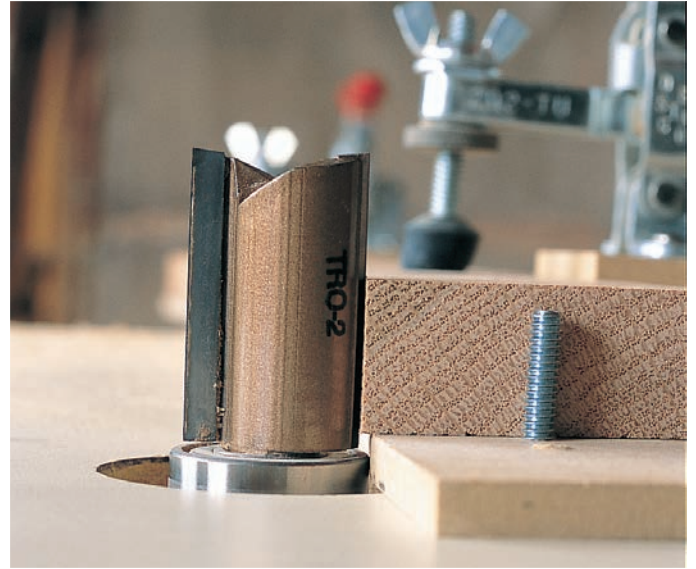
An offset pattern bit takes the worry out of sawing close to the contour line traced from your template. If you saw to within \frac{1}{8} " or \frac{3}{16} " of it, you're fine. Guide the template and work along the offset pattern bit to trim a manageable amount of the excess, leaving \frac{1}{16} " to be trimmed on the final pass with a flush bit.
