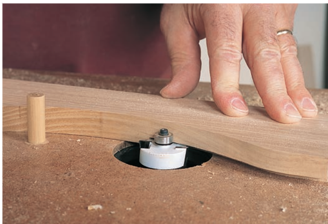
While the rabet bit has some limitations, it is easy to set up, cutting predictable widths without time-consuming test cuts. Rabbeting curved work is something only a piloted rabet bit can do.
