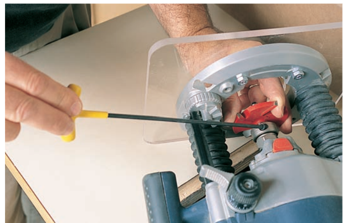
A great accessory that fits selected router brands and models is the Eliminator RC chuck. It enables you to change bits in seconds with a hex-key wrench. No need to hold a spindle lock or fumble with an open-end wrench. Hold the bit in one hand and twist the hex key to tighten the collet with the other.
