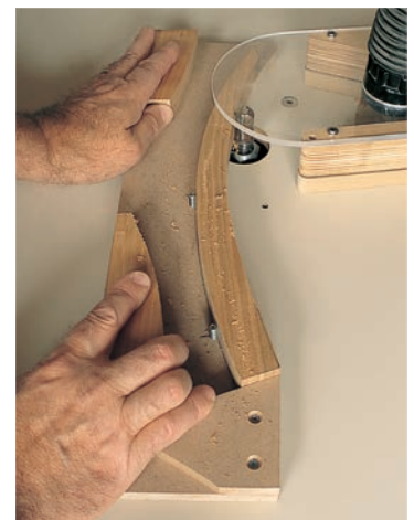
Making a batch of small parts safely often requires more than one template. The small curved slat shown (left) is a good example. The slat is too slender to be routed using a rout-around template. But you do need a pattern to lay out the slat blanks, and making that pattern from hardboard rather than cardboard simplifies making the working templates. Use it to make a convex template (center) and a concave template (right). Band-saw a slat blank and stick it to the convex template with carpet tape. Position fences—they need only contact the blank at three places to locate it—and attach them to the template. After shaping the blank's convex edge, stick it to the concave template. Mount fences (machine screws are used here) to locate the blank. Rout the concave edge. (The extra blocks attached to the templates are scraps of the working stock; they allow the templates to be inverted and used with a flush-trimming bit.)
