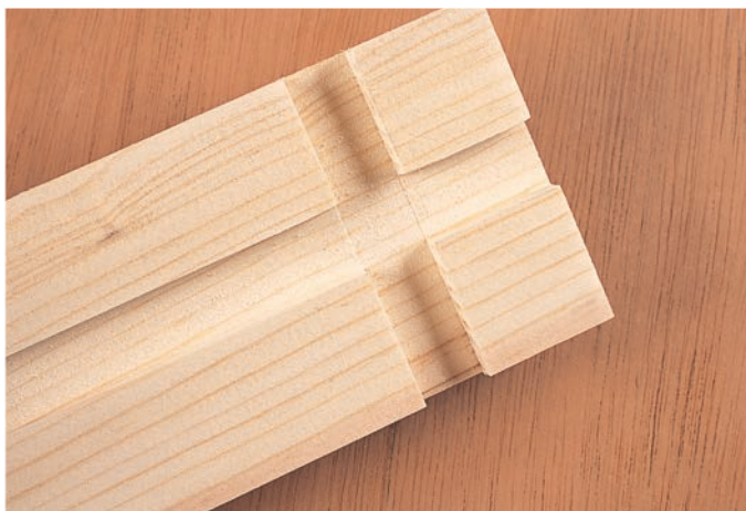
One is a dado, and one is a groove. Both were cut with the same bit. The cross-grain cut is the dado, the long-grain cut is the groove.
