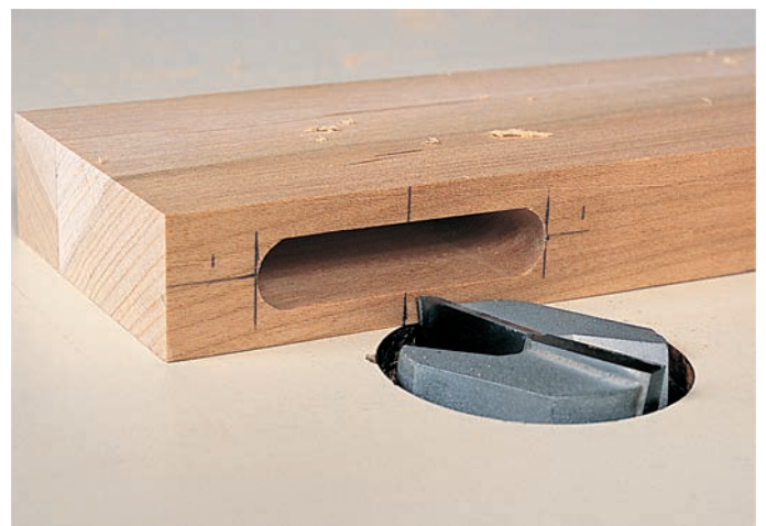
Use a finished part as a gauge to set a bit for cutting its mate. So to cut a tenon that'll fit this mortise, set the bit's tip flush with the mortise's cheek. The same technique works for other joints, including the tongue-and-groove and cope-and-stick.
